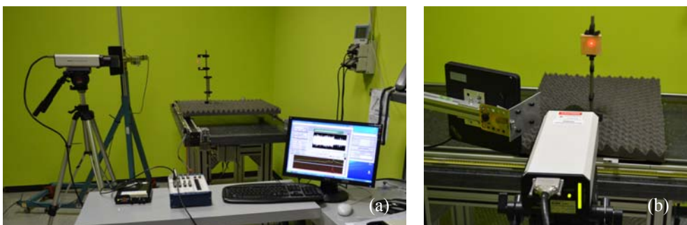
FIG.6: The laboratory equipment for LDV measurements (a); the HAS8 – sample – LDV configuration (b).
